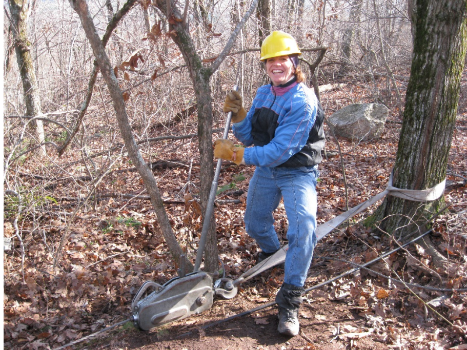
Pat operating the grip hoist on Wachusett Mountain (photo courtesy of Claude Guerlain)
